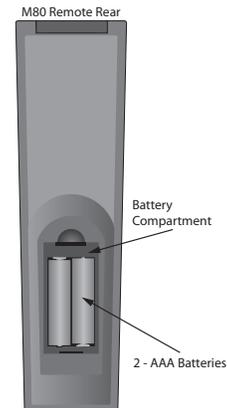
**Diagram 77** Installing M80 Remote Control Batteries
