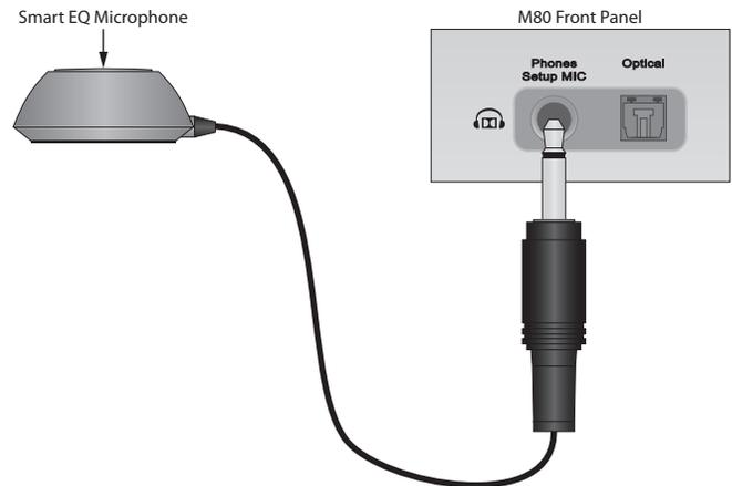
**Diagram 46** SmartEQ Microphone Connection
