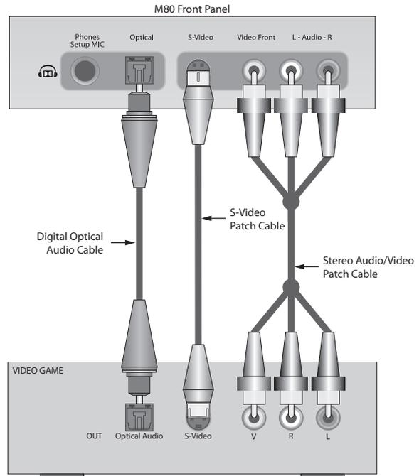
**Diagram 26** Front Panel A/V Connections
