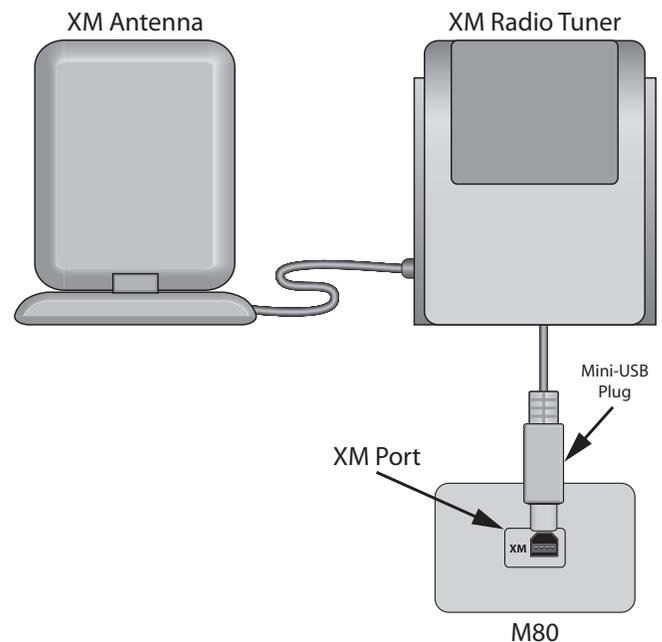
**Diagram 10** XM Tuner Connections
