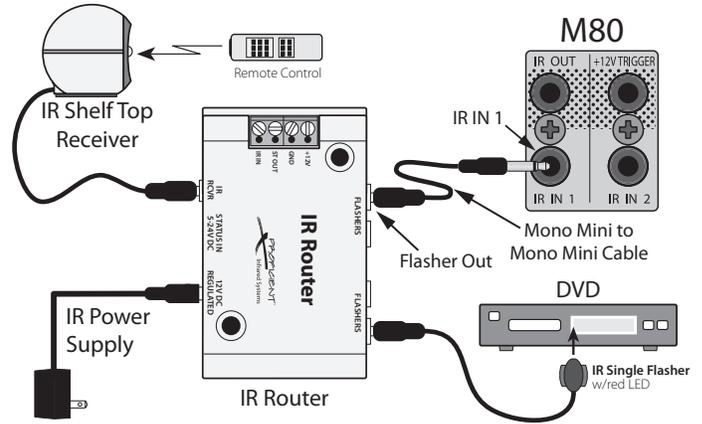
**Diagram 21** IR IN Connections with IR Flashers
