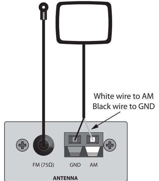
**Diagram 9** Antenna Connections
