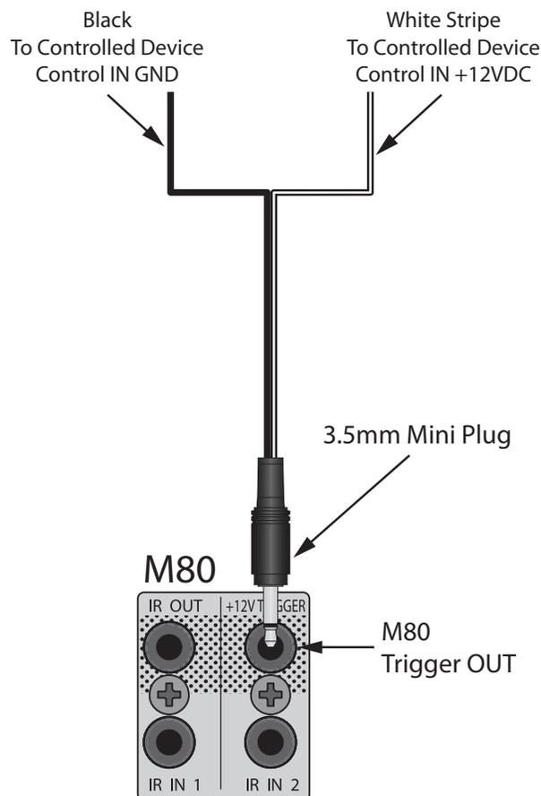
**Diagram 20** Trigger Out Connections
