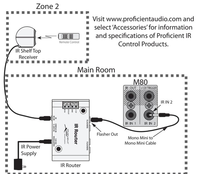
**Diagram 124** Zone 2 IR Control Connections
