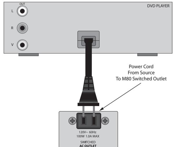
**Diagram 24** Switched Outlet Connections
